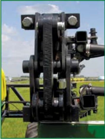
WIDE-BUSHED PINS FOR EXTENDED HINGE LIFE.
